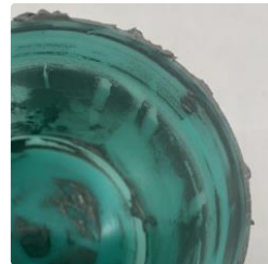
After using the perforated pot type automatic solder supply
