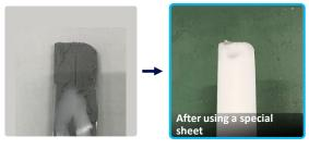
**Solder remaining in the perforated pot** when automatic solder supply is used
