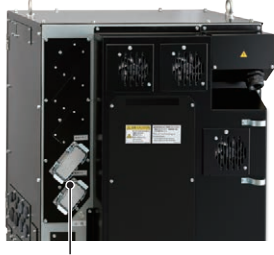
M-C/built-in external axis cables arranged on the back
