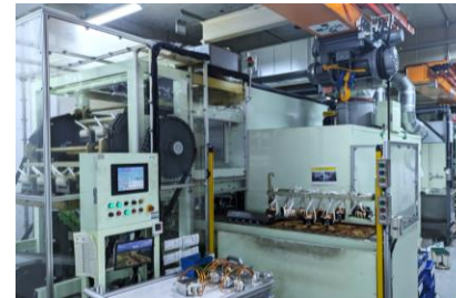
New varnish impregnation and drying equipment
