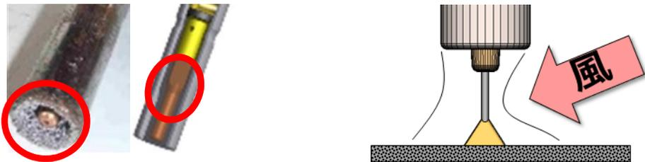
The diagram illustrates two scenarios. On the left, a close-up of a welding nozzle shows spatter (red circles) and a damaged orifice. On the right, a cross-section of a weld shows air flow (indicated by a red arrow labeled '風') entering the weld pool from the side, causing defects.
