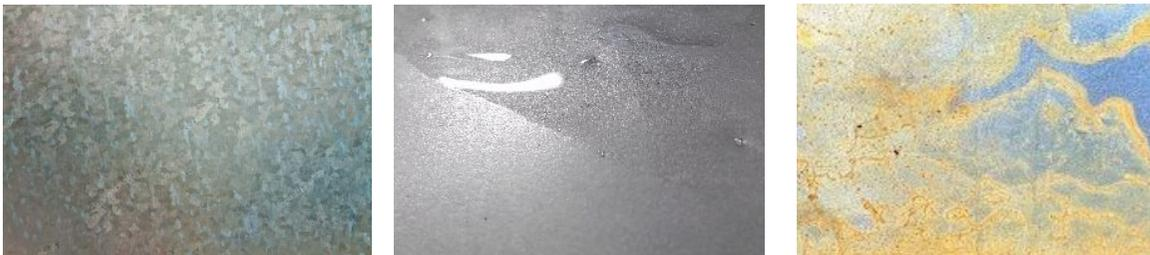
Three photographs show different surface contaminants: zinc plating (left), mechanical oil (middle), and rust (right).
