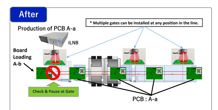
PCBs that are different from those in production are suppressed from being brought into the machine after detection at a gate in the line.
